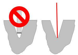
The CCMP beam allows you to search for reversal points in extremely small areas not accessible to a contact sensor.
