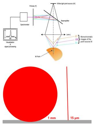
The beam of the CCMP sensor is extremely small compared to a 1 mm ball. Furthermore, there is no influence due to material deformation during measurement. A chromatic lens L generates the image of a point source of white light W as a continuum of monochromatic images located on the optical axis ("chromatic coding").
