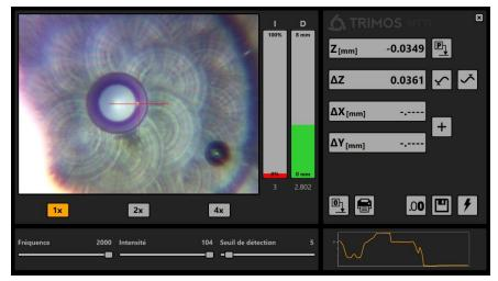
The **Trimos Compact Z** software is extremely simple. Its philosophy is inspired by the philosophy of the height gages that have made Trimos so successful. It allows quick noncontact height measurements even for inexperienced users.
